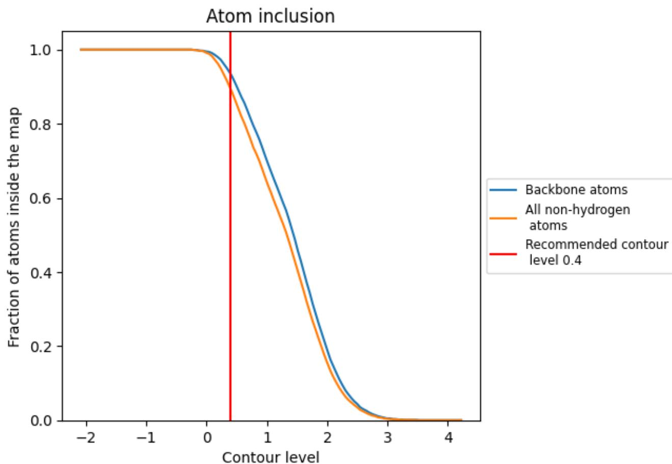
At the recommended contour level, 93% of all backbone atoms, 89% of all non-hydrogen atoms, are inside the map.
